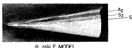
Fig. 5 Surface flow on 10^\circ cone; M = 2 ; \alpha = 15^\circ .
