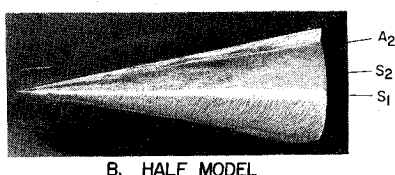
Fig. 6 Surface flow on 10^\circ cone; M = 2 , \alpha = 30^\circ .
